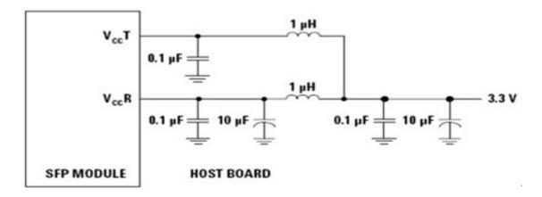
Note: Inductors with DC resistance of less than  $1\Omega$  should be used in order to maintain the required voltage at the SFP input pin with 3.3V supply voltage. When the recommended supply filtering network is used, hot plugging of the SFP transceiver module will result in an inrush current of no more than 30 mA greater than the steady state value
