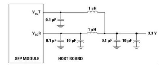
Note: Inductors with DC resistance of less than  $1\Omega$  should be used in order to maintain the required voltage at the SFP input pin with 3.3V supply voltage. When the recommended supply filtering network is used, hot plugging of the SFP transceiver module will result in an inrush current of no more than 30 mA greater than the steady state value
